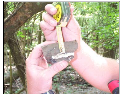
Measuring sediment deposited in a backswamp area after flood season.
