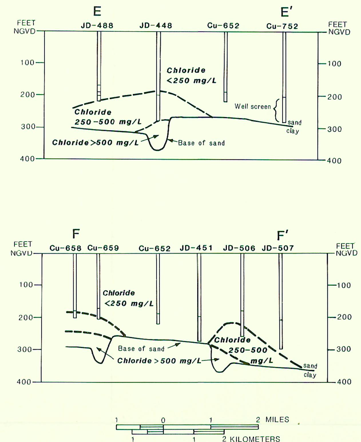
Cross sections showing variation in chloride concentration in relation to location of the channel in the base of the "upper sand" in the vicinity of the town of Iowa
