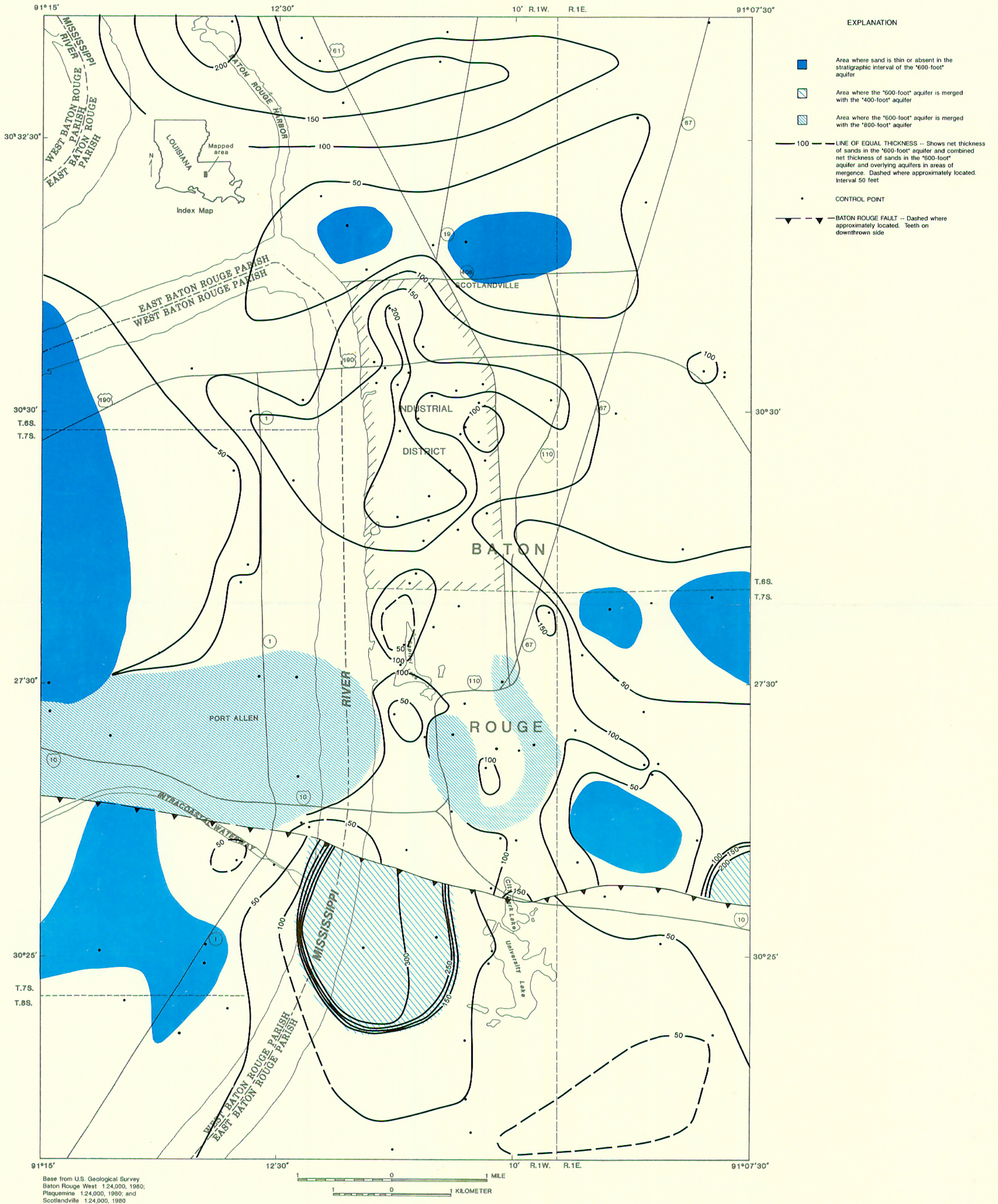
PLATE 19. NET SAND THICKNESS OF THE "600-FOOT" AQUIFER IN THE BATON ROUGE INDUSTRIAL DISTRICT AND THE SURROUNDING AREA, LOUISIANA.
