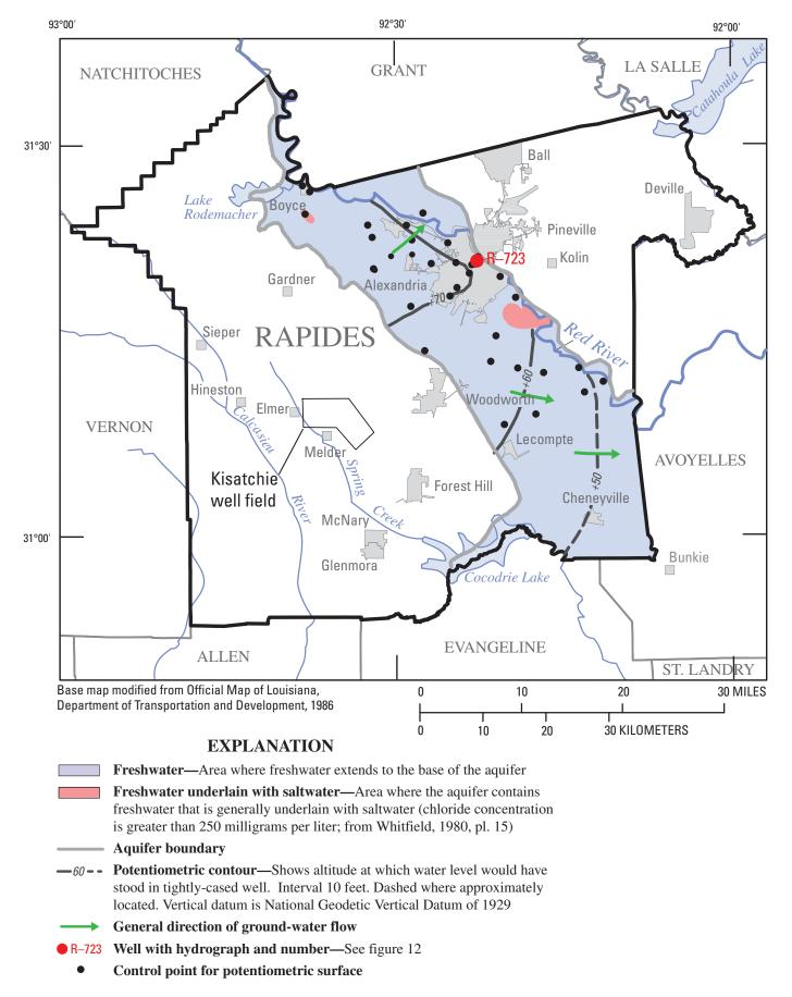
Figure 11. Generalized potentiometric surface of the River River alluvial aquifer in Rapides Parish, Louisiana, July 2000.
