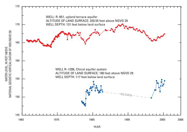
**Figure 17.** Water levels in wells R-851 and R-1208, screened in the upland terrace aquifer and Chicot aquifer system, in western Rapides Parish, Louisiana (see figure 16 for well locations).
