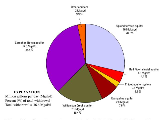
**Figure 3.** Water withdrawal by aquifer or aquifer system in Rapides Parish, Louisiana, 2000 (B.P. Sargent, U.S. Geological Survey, modified written commun., 2002).
