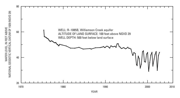
**Figure 28.** Water levels in well R-1085B screened in the Williamson Creek aquifer in Rapides Parish, Louisiana, See figure 27 for well location.
