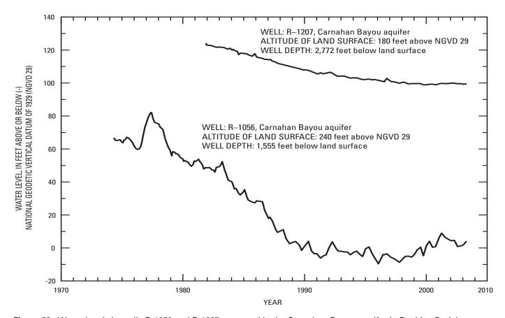
**Figure 33.** Water levels in wells R-1056 and R-1207 screened in the Carnahan Bayou aquifer in Rapides Parish, Louisiana. See figure 32 for well location.
