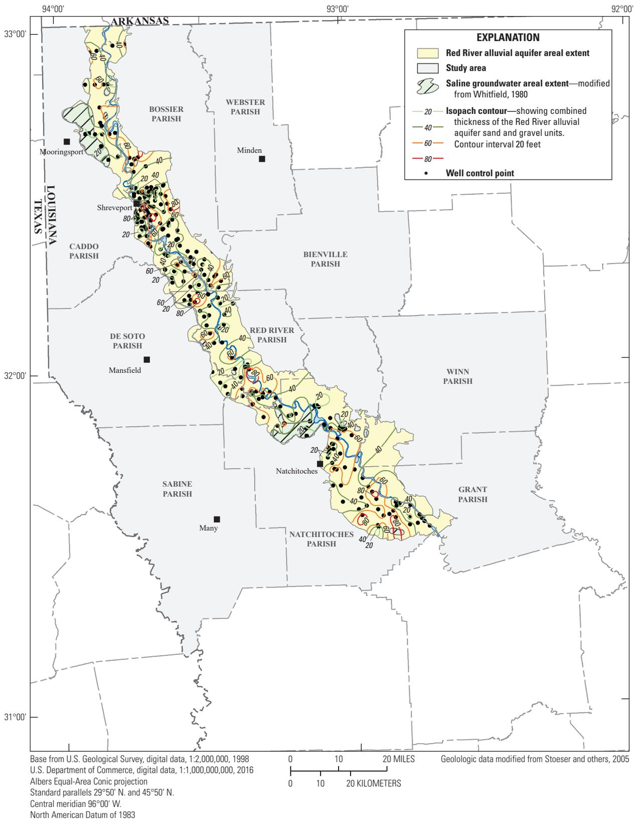
**Figure 4.** Combined thickness of the sand and gravel unit and areas of saltwater in the Red River alluvial aquifer in northwestern Louisiana.
