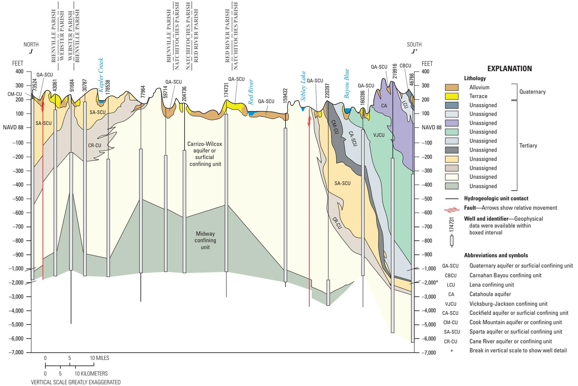
Figure 14. Hydrogeologic cross section J-J' and base of freshwater water-quality zone in northwestern Louisiana.
