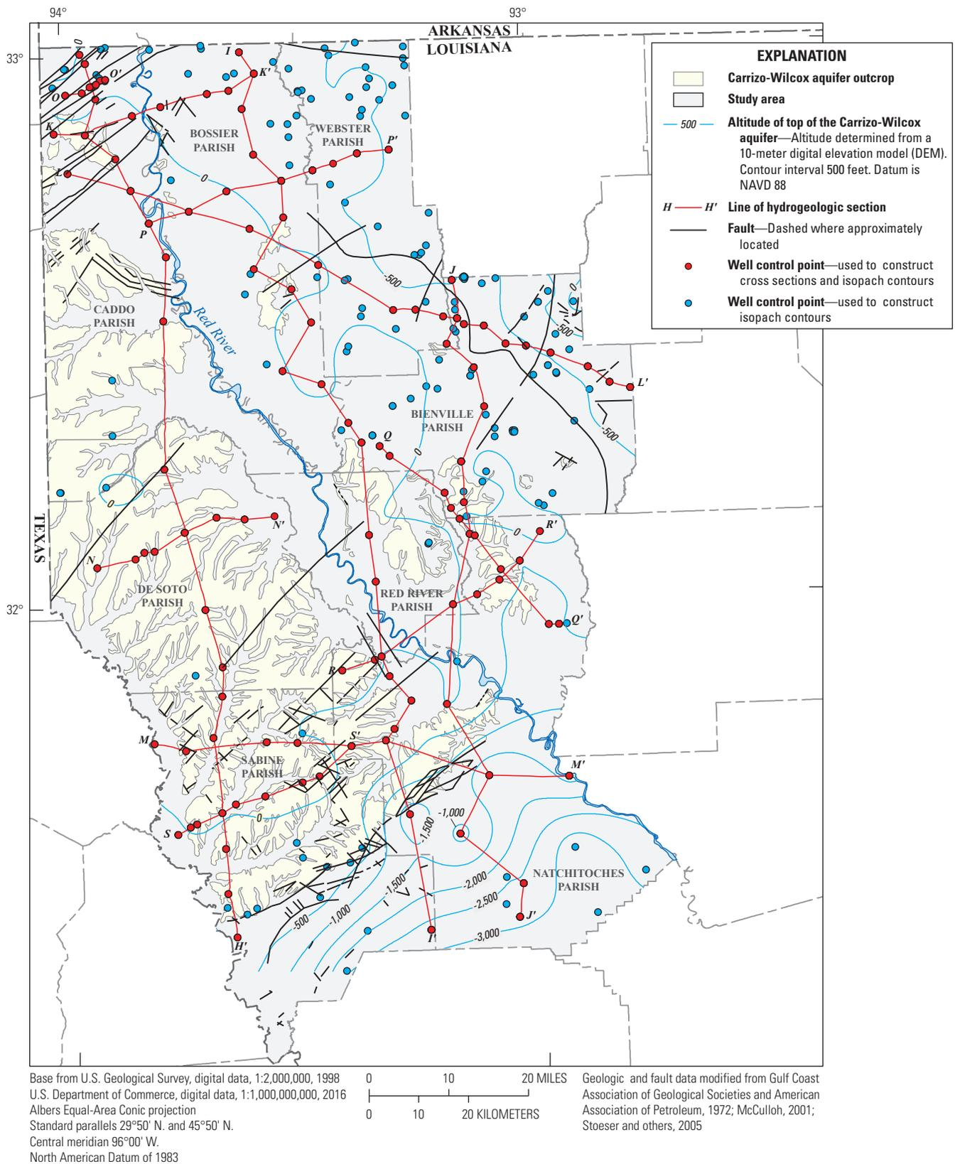
**Figure 25.** Outcrop area and altitude of the top of the Carrizo-Wilcox aquifer and lines of hydrogeologic cross sections  $H-H'$  through  $S-S'$  in northwestern Louisiana.
