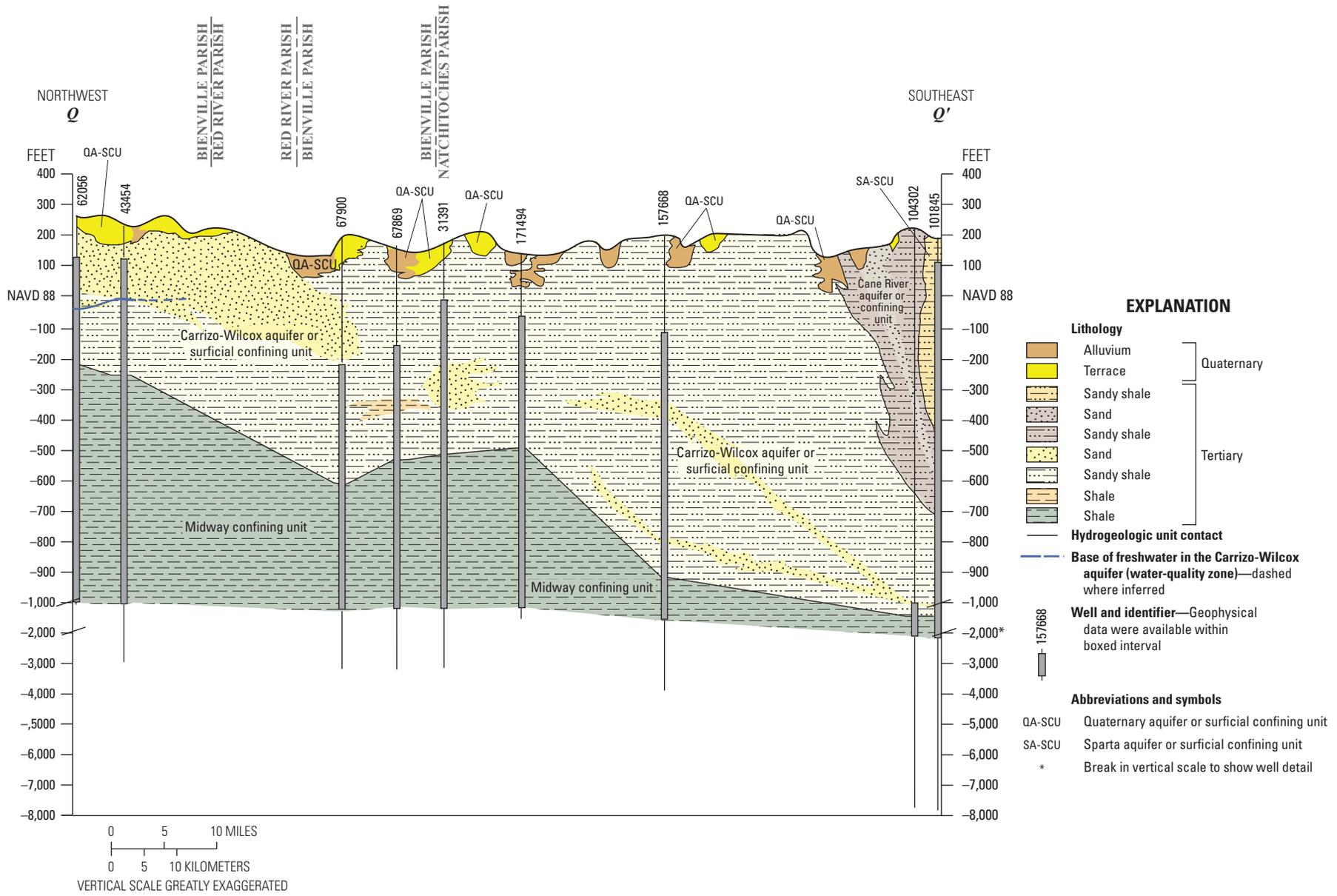
**Figure 21.** Hydrogeologic cross section  $Q-Q'$  and base of freshwater water-quality zone in northwestern Louisiana.
