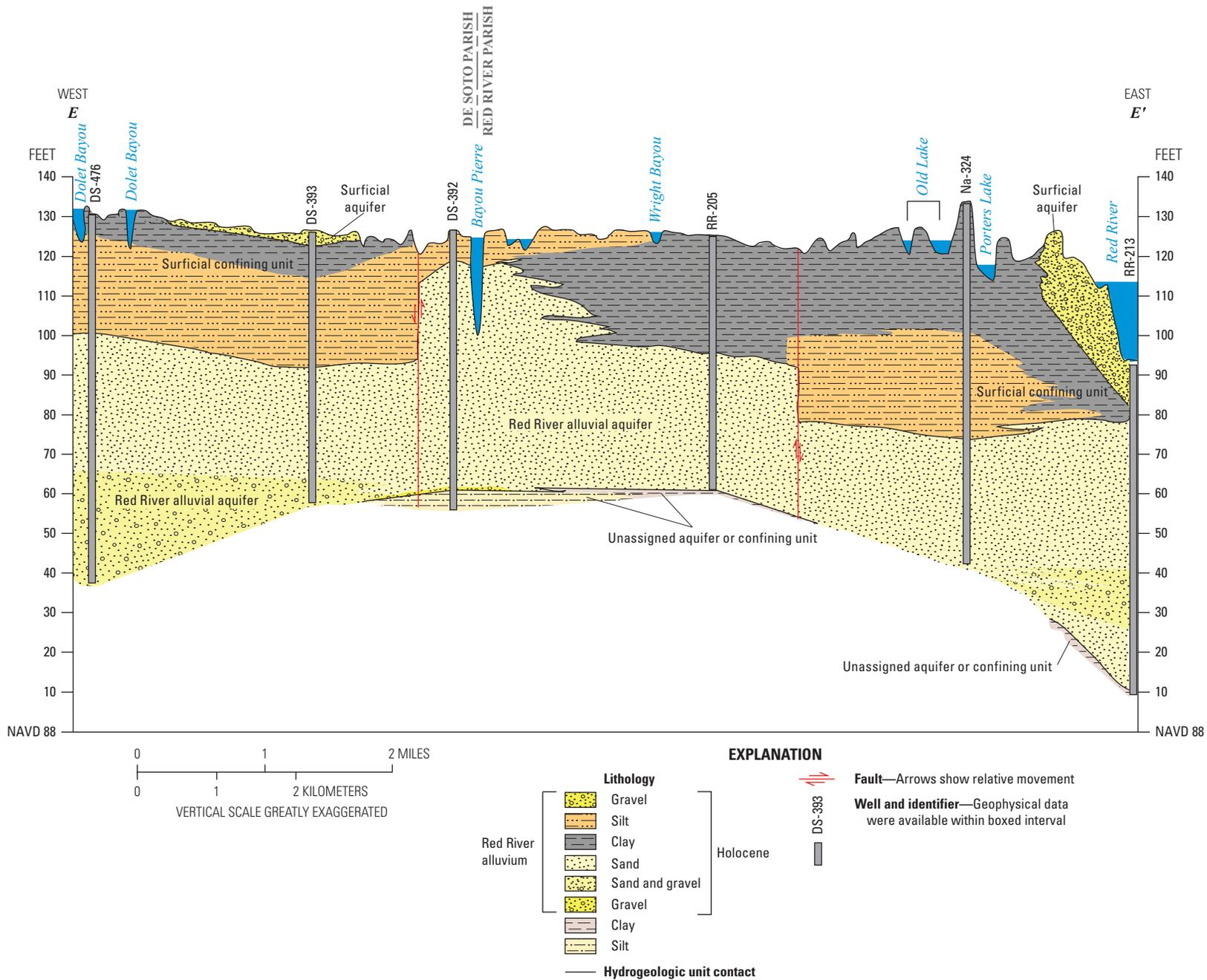
**Figure 9.** Hydrogeologic cross section E–E' of the Red River alluvial aquifer in northwestern Louisiana.
