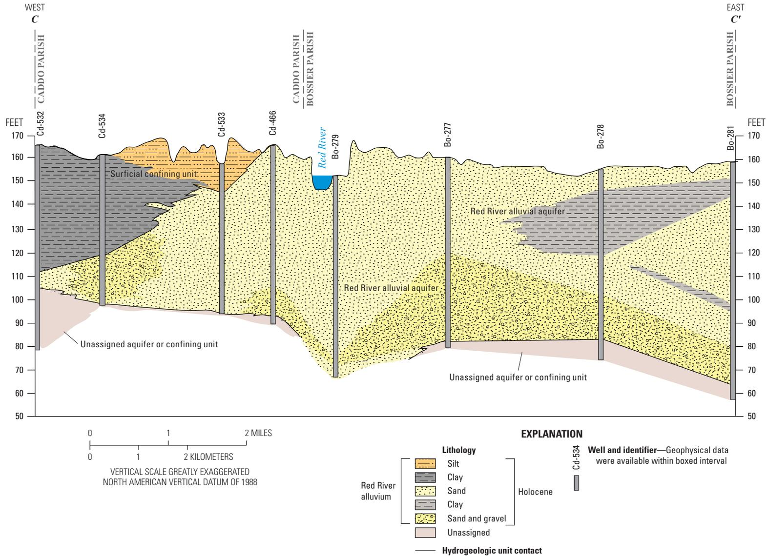
Figure 7. Hydrogeologic cross section C–C' of the Red River alluvial aquifer in northwestern Louisiana.
