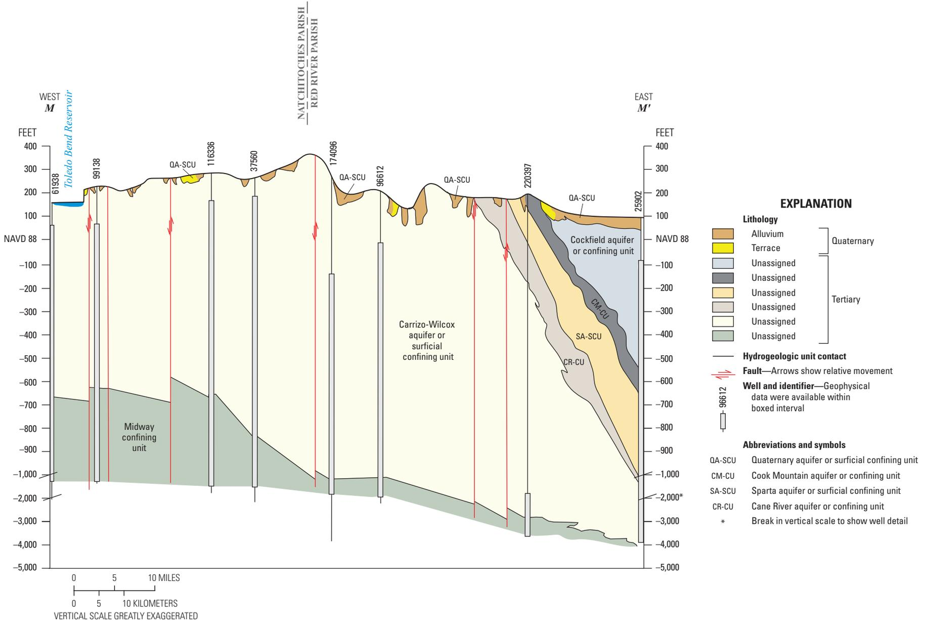
Figure 17. Hydrogeologic cross section *M-M'* and base of freshwater water-quality zone in northwestern Louisiana.
