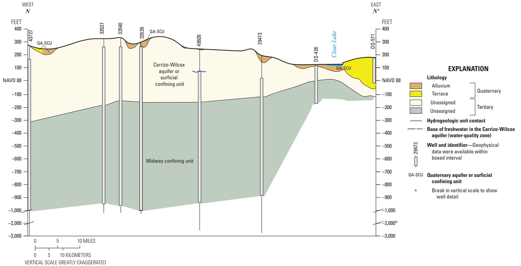
**Figure 18.** Hydrogeologic cross section  $N-N'$  and base of freshwater water-quality zone in northwestern Louisiana.
