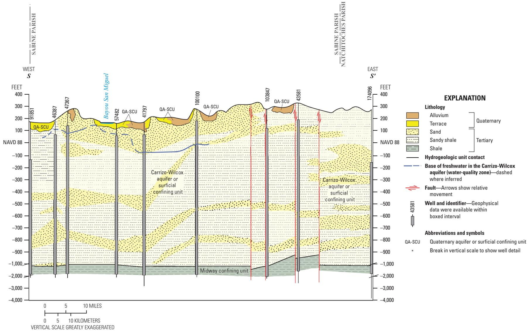
Figure 23. Hydrogeologic cross section S-S' and base of freshwater water-quality zone in northwestern Louisiana.
