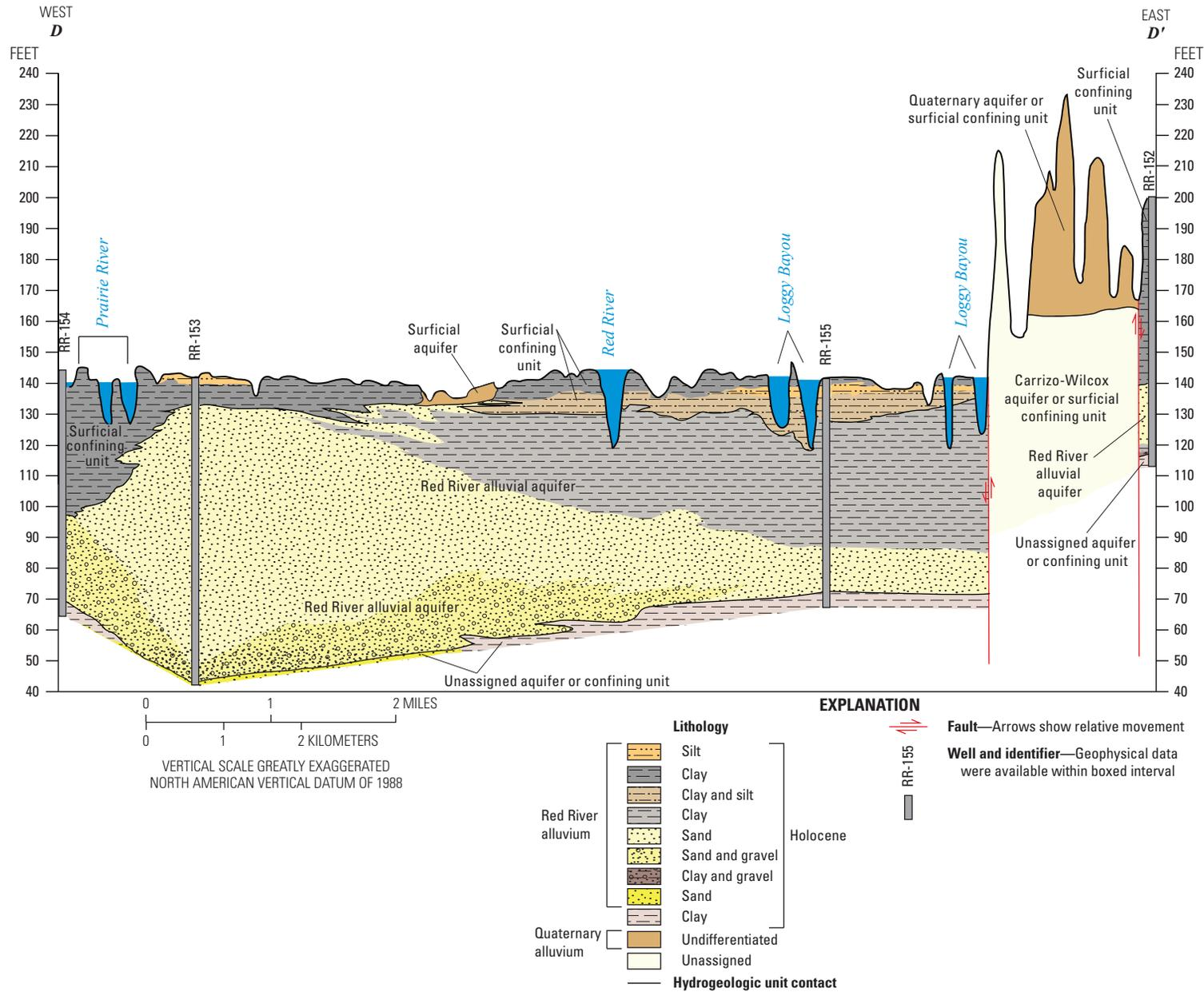
Figure 8. Hydrogeologic cross section D–D' of the Red River alluvial aquifer in northwestern Louisiana.
