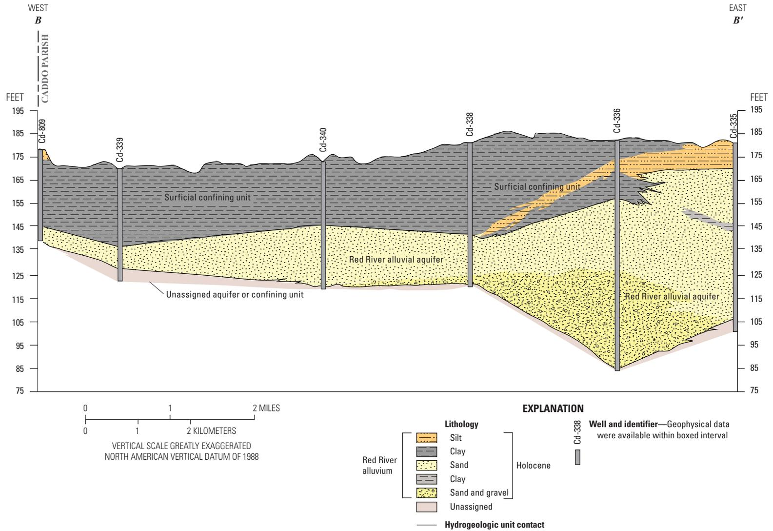
**Figure 6.** Hydrogeologic cross section *B–B'* of the Red River alluvial aquifer in northwestern Louisiana.
