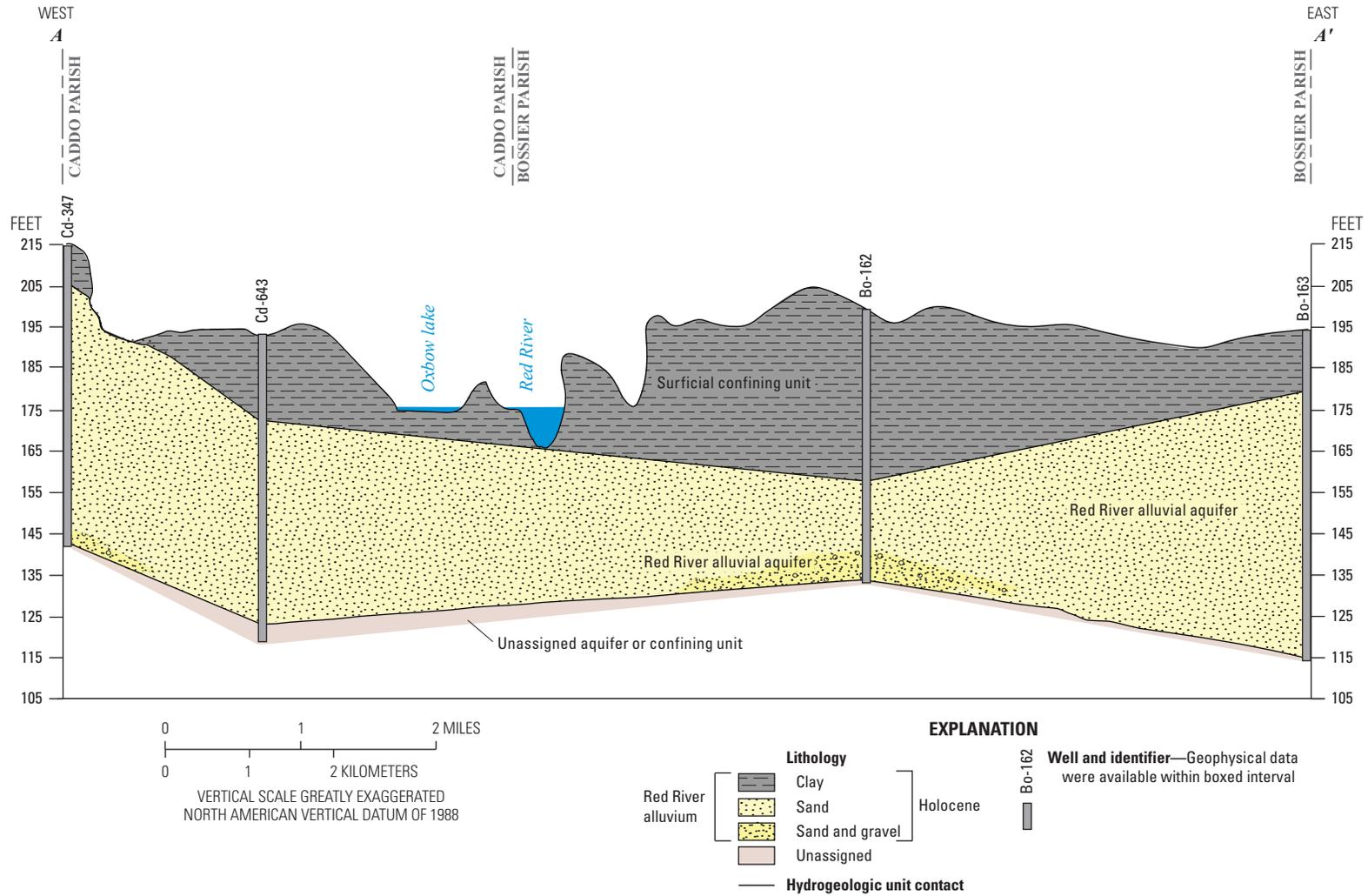
Figure 5. Hydrogeologic cross section A–A' of the Red River alluvial aquifer in northwestern Louisiana.
