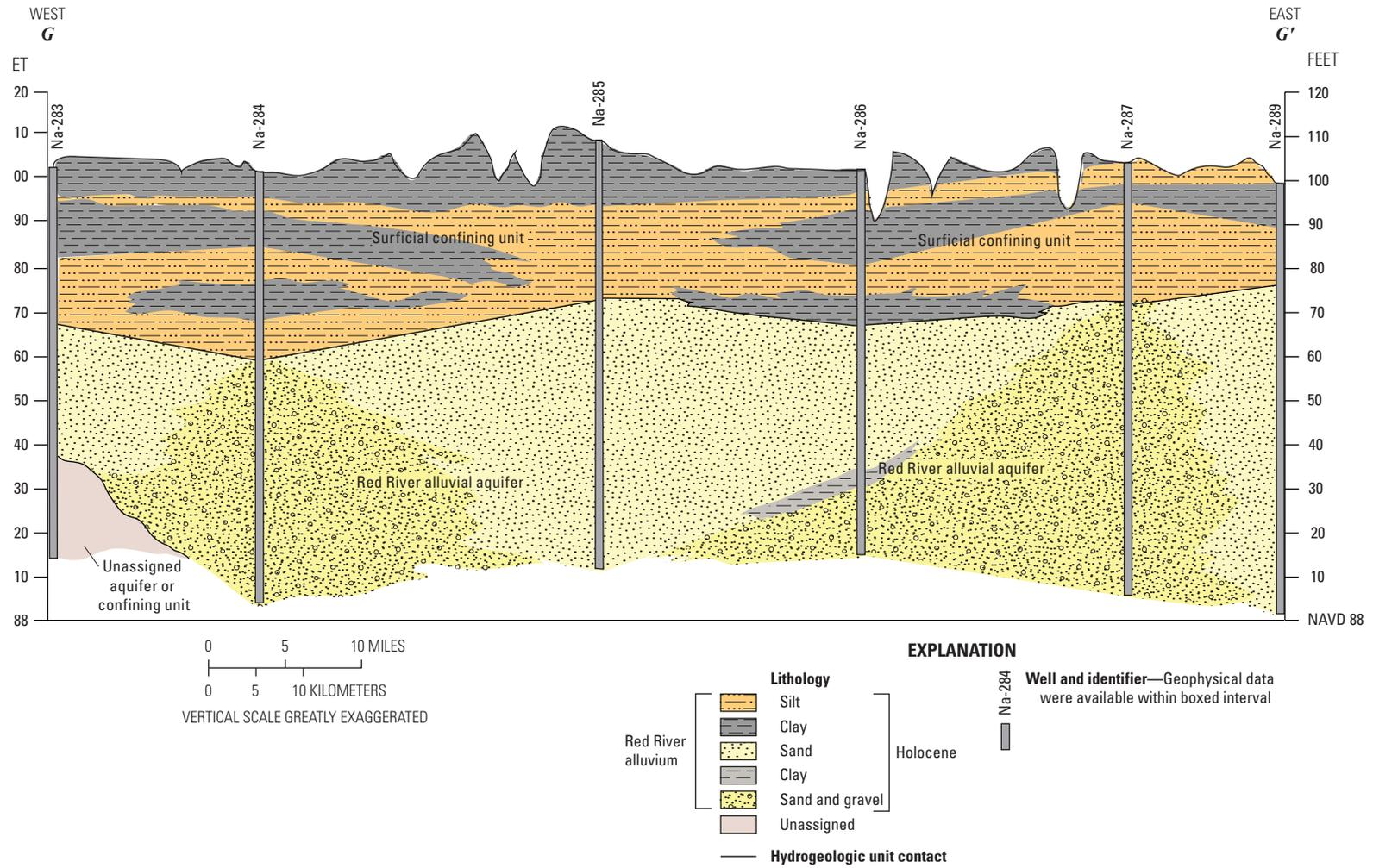
Figure 11. Hydrogeologic cross section G–G' of the Red River alluvial aquifer in northwestern Louisiana.
