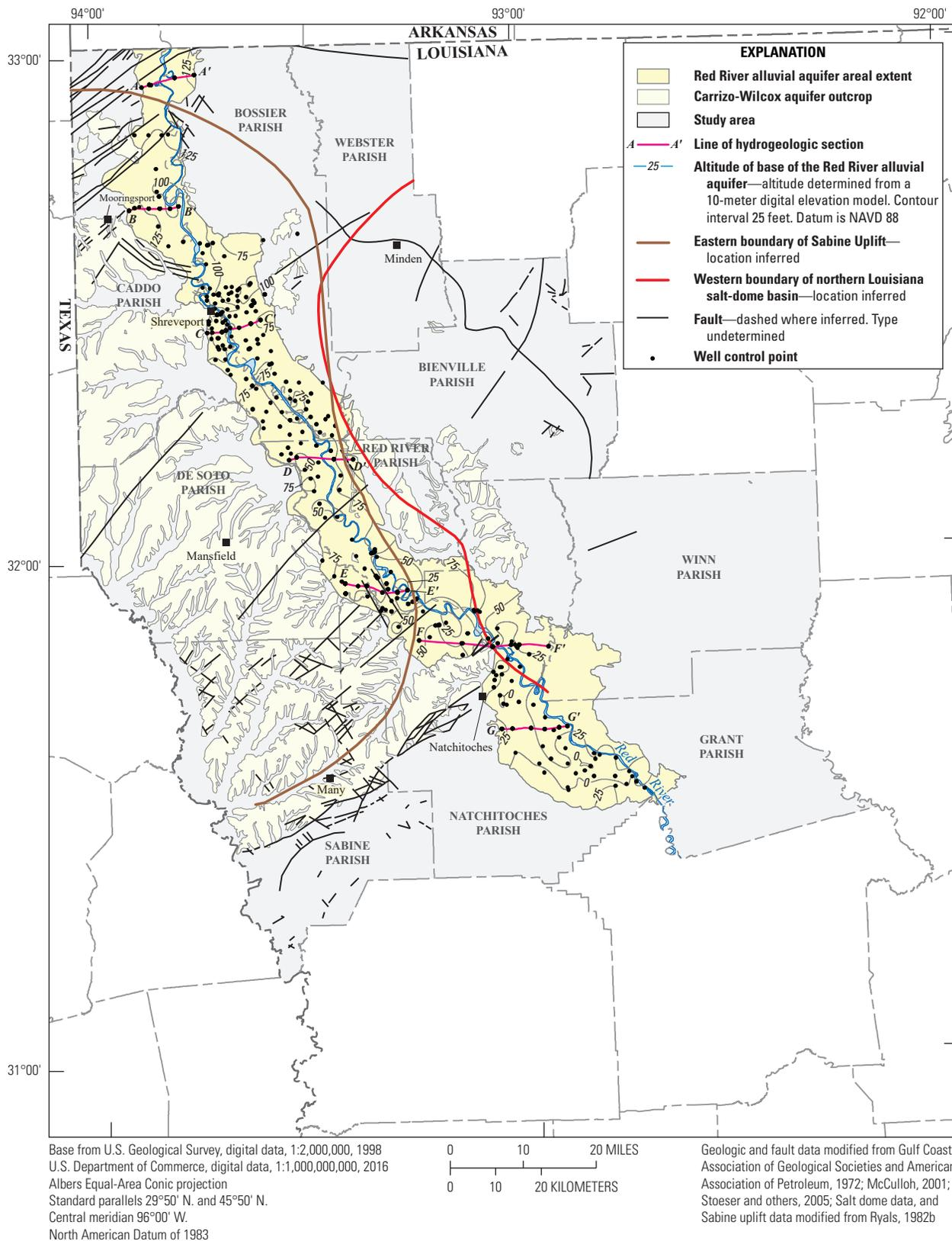
**Figure 3.** Altitude of the base of the Red River alluvial aquifer, extent of principal aquifers, and lines of hydrogeologic sections A–A' through G–G' in the Red River valley in northwestern Louisiana.
