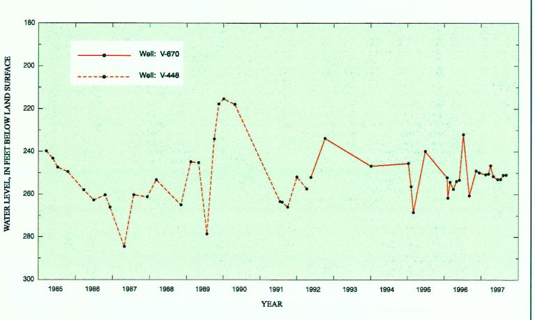
**Figure 8.** Water level in well V-448 and replacement well V-670 completed in the Williamson Creek aquifer "B" sand at Fort Polk cantonment, 1985-97.
